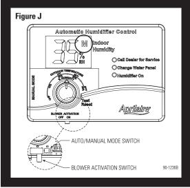
**NOTE:** If control setting was changed between Automatic and Manual mode, power to the control must be cycled by removing then reinstalling the R wire.
