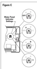
**Set to "OFF"** for Model 800 Series humidifiers or to turn the Humidifier Pad Change indicator to off.
