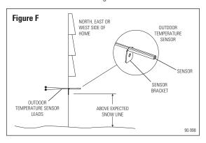
**NOTE:** A convenient way to get the sensor wire outside is to make use of unused wires running to the A/C condensing unit (if applicable). Other ways are to use existing holes for cable TV lines, telephone lines, A/C lines, etc. Read all equipment instructions beforehand for possible conflicts and warnings.
