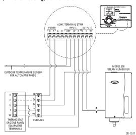
\*Model 700 Series humidifiers produced prior to October 2007 have an almond color housing and internal transformer providing 24VAC to the solenoid valve. Models produced after October 2007 have a gray housing and external transformer provided with the unit. For zoned HVAC systems, refer to the THERMOSTAT IN A ZONED HVAC SYSTEM section found in the Series 800 Steam Humidifier Installation and Maintenance Instructions for instructions pertaining to ductwork and wiring.
