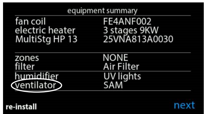
Fig. 2 – Ventilator Properly Discovered
