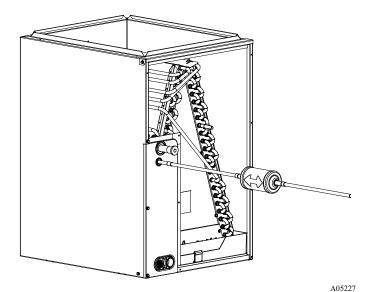
Fig. 25 - Liquid Line Filter Drier - HP
