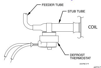
Fig. 8 – Defrost Thermostat Location
