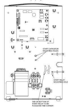
Fig. 43 – Start Relay and Capacitor Mounting Locations in Cube Cabinet
