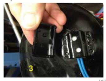
4. Slide out the sensor, slide in replacement and reinstall the cover
