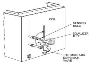
Fig. 28 - Typical TXV Installation
