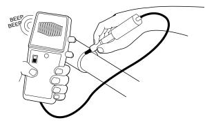
Fig. 29 - Electronic Leak Detection
