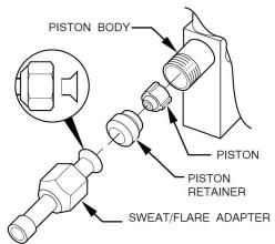
Fig. 21 – AccuRaterr Components (used in R-22 Heat Pumps)
