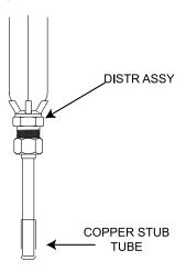
Fig. 34 – Copper Stub Tube Connection
