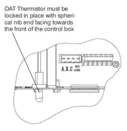
Fig. 45 – Outdoor Air Thermistor (OAT) Attachment
