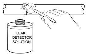
Fig. 30 - Bubble Leak Detection
