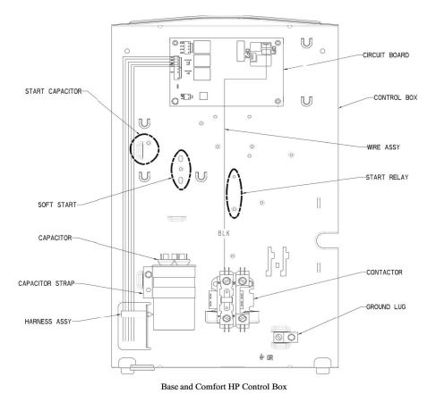
Fig. 3 – Legacy Series Control Box Identification
