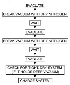
Fig. 36 - Triple Evacuation Method
