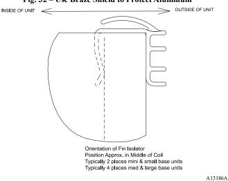
Fig. 33 - Fin Isolator Orientation
