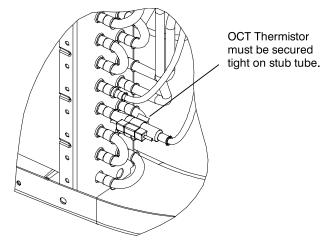
Fig. 46 - Outdoor Coil Thermistor (OCT) Attachment
